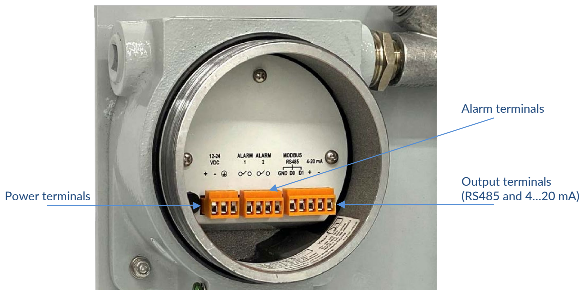
Figure 4. Wiring and connection (AIS models)
