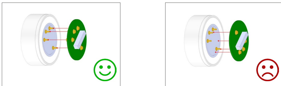
Figure 24. Aligning your sensor and PCB
