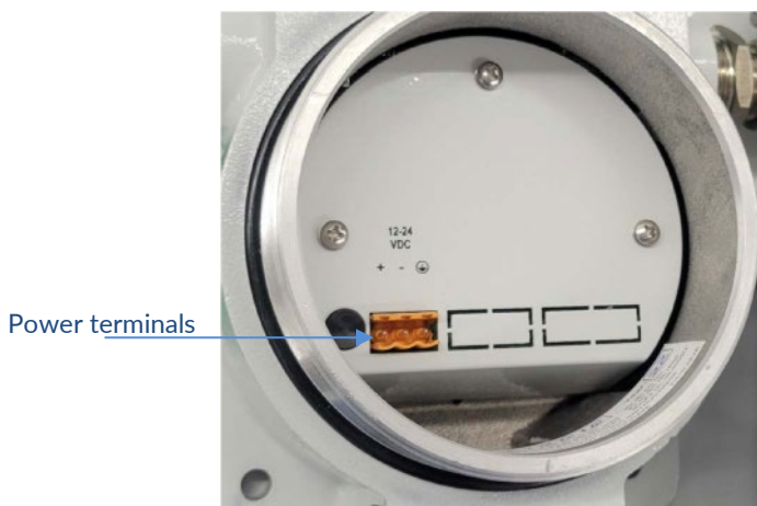
Figure 3. Wiring and connection (IS models)
